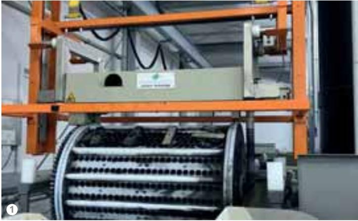
**Figure 1: Dörken MKS-Systeme developed a bulk cataphoresis process called DELTA-eLACK® with a drum system.**
