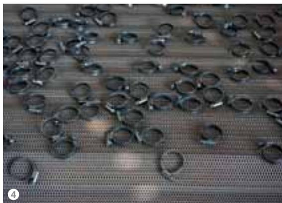
**Figure 4: The workpieces are transferred from the conveyor belt to a drum that is rotated and immersed in the tank containing the cathaphoresis product.**
